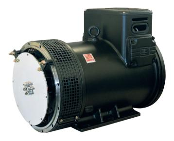
The auxiliary winding is responsible to provide independent power for the voltage regulator under all sorts of load, with no electrical link to the main winding. This way, load application, rejection or any other variation will not impact the power input for the voltage regulator. WEG's auxiliary winding ensures 300% of short circuit current up to 10 seconds.
