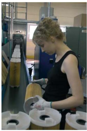
At the end of the production process a visual inspection ensures that only perfectly produced filters are delivered to the customer.
