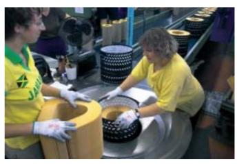
Inserting the filter bellows in the housing
