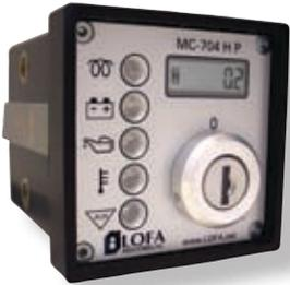
The MC704HP is a compact micro panel with imbedded high current key switch and LED hour meter for diesel engine control, monitoring, and protection featuring LOFA's First-Fault Diagnostics (FFD) and automatic preheat control. FFD monitors battery charge, low oil pressure, high temperature, and one additional auxiliary contact closure input. The MC704LCP is available for applications that do not require an hour meter.
