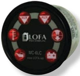
The MC6LC is a compact micro indication instrument for mechanically governed diesel engine monitoring and installs into 2" (52mm) gauge openings. It works well for low cost applications not requiring engine shut down protection. Bright LED illuminated symbols monitor battery charge, low oil pressure, high temperature, air filter restriction, and two auxiliary contact closure inputs.
